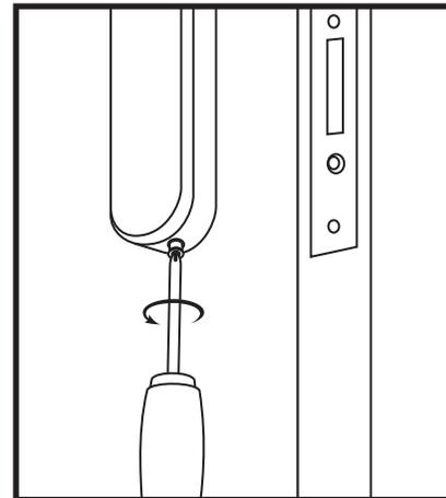
**9** Turn the screw at the bottom of the inner handle set anti-clockwise (go outside) until you feel resistance.
