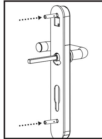
**4** Screw two fixing poles on the outer handle set.
