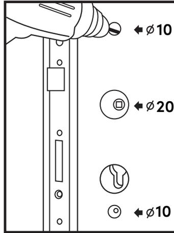
**2** Drill the holes on the door according to the Door Drilling Template.
