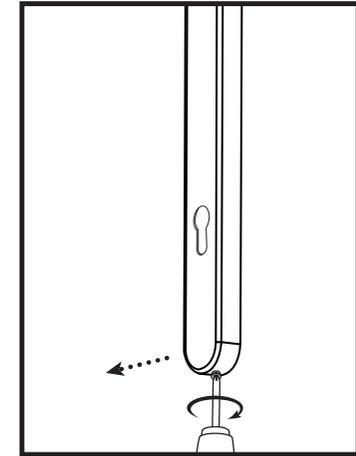
**6** Turn the screw at the bottom of inner handle set clockwise (go inside) until the cover plate can be pulled out.
