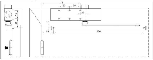
Provided the structural conditions allow, an opening angle of 180° is possible with this method of fixing.
