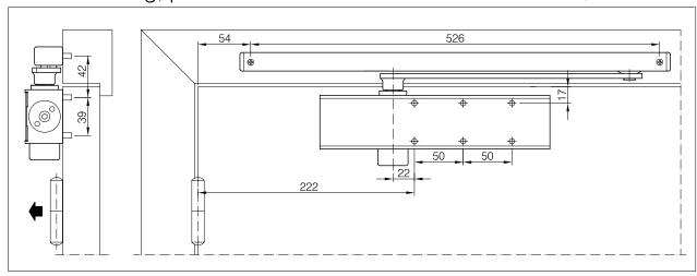
Provided the conditions allow, an opening angle of 180° is possible with this method of fixing. In most cases, however, a wall recess will have to be provided for the door closer.
