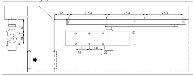
Depending on the structural conditions, the door opening angle with this method of fixing is limited to approx. 160°.
